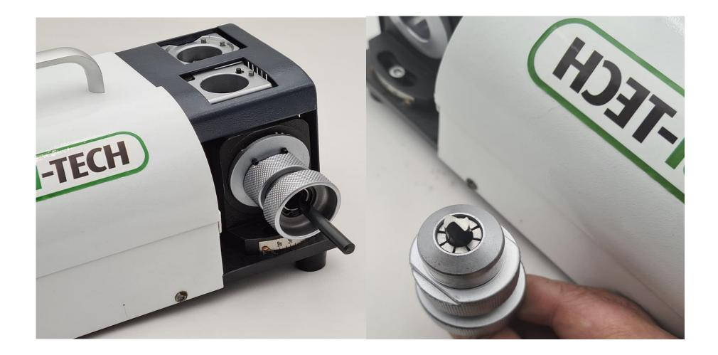
3 After motor start-up. Place the chuck in the grinding base, taking care to position the flat of the chuck with the two small locating pins (as shown in the picture). Press lightly on the grinding wheel with a smooth, continuous movement, turning clockwise until there is no grinding noise. Then remove the chuck and repeat the operation, rotating the assembly through 180° to sharpen the other cutting edge.
