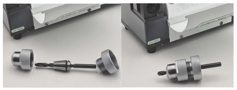
1 Select the collet with the clamping tolerance that corresponds to the diameter of the drill to be sharpened and proceed with assembly as shown in these 2 images.
