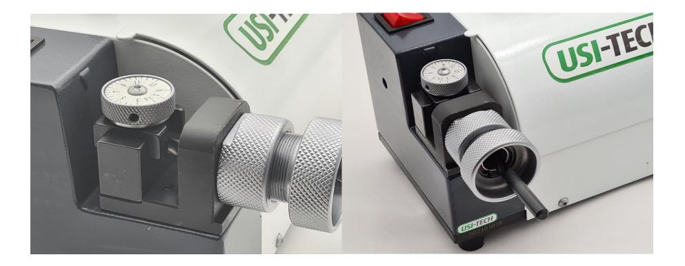
2. Adjust the sharpening positioning finger by positioning the sharpening diameter to be sharpened.
